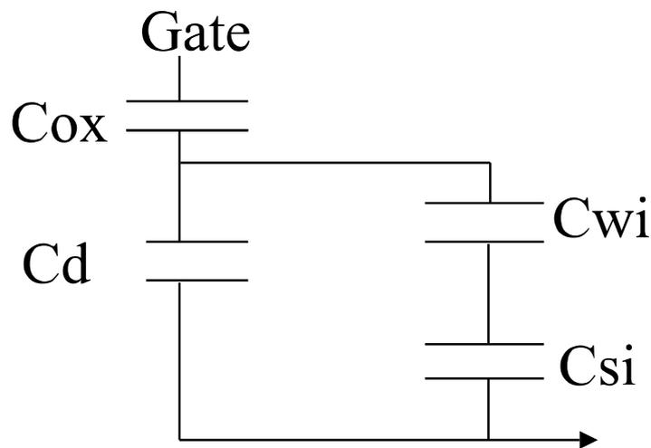
Fig. 3: Equivalent circuit of a MOS capacitor under inversion conditions.
