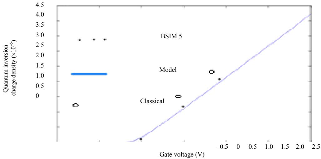
Fig. 2: Simulated results of quantum mechanical inversion charge density with gate voltage under the model parameters: substrate doping  $1 \times 10^{18} \text{ cm}^{-3}$  and oxide thickness 1.5 nm.
