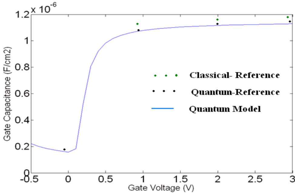
Fig. 4: Simulated results of the quantum gate capacitance. The green dots show the classical gate capacitance and the black dots show the reported [14] quantum mechanical gate capacitance. The blue line shows the modeled quantum mechanical gate capacitance.
