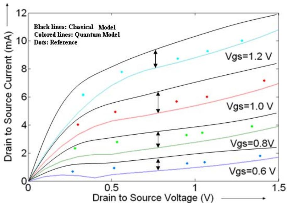
Fig. 4: Simulated drain current at channel length ( $L$ )=80nm (Gate length ( $L_g$ )=130nm) including inversion layer quantization, poly silicon gate depletion, DIBL and mobility reduction at gate doping  $N_p = 10^{19} \text{ cm}^{-3}$  and  $V_{bs}$  (body bias) = -0.75. (Empirical fit of 0.03 V has been given to account for polysilicon depletion effect). The colored dots show the reported results [19]. The black lines show the classical modeled results.
